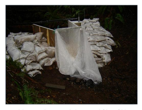
We sampled macroinvertebrate export at the downstream end of the non-fish-bearing stream basins every six weeks over a 24-hour period using a 250-micron drift net.
