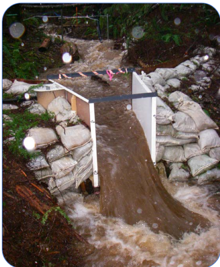
Measuring discharge and suspended sediment at the outlet of a headwater basin.
